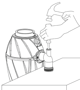
Removal of the diaphragm
