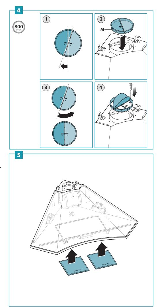
EN - Reassemble the metallic filters.
