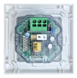
• **Mounting holes.** The mounting holes are used to screw the module into a flush mounting box.
